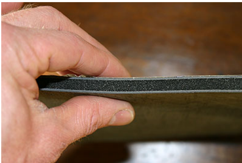
8 mm thick sandwich construction
