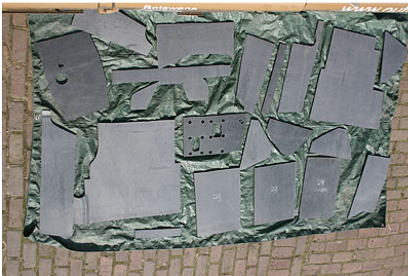
Arial view of all the pieces of the front cab kit. Note the in the center the precut part to be fitted to the bulkhead panel around the pedals (picture above)
