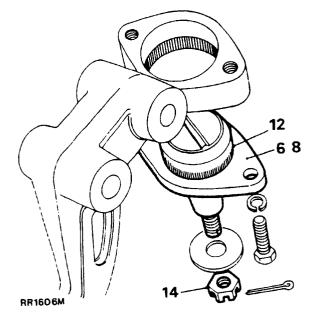
14. Fit the pivot bracket complete with ball joints to the rear axle. Tighten to the correct torque (see section 06-Torque values).
