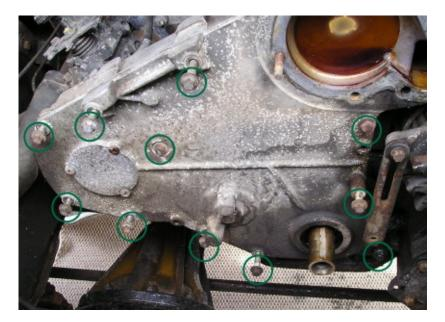
Then loosen the timing case cover , I do this leaving all the bolts in place as there are three different lengths so its easy to get confused putting them all back together.
