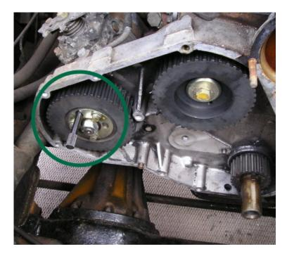
Now you must do set the timing. I had difficulty setting the injector pump timing as some cowboy had been there before me and I couldn't get the pin in (above picture), so I cut the belt off and started to line it all up properly.
