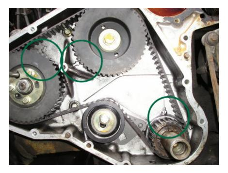
This is what we need to do. (picture above) Bottom right is the crankshaft, that woodruff key (little square notch on top of crank) sits at 12 o'clock in line with the arrow above it. Lock this in place by putting a locking pin in the flywheel housing drain plug (next picture below).
