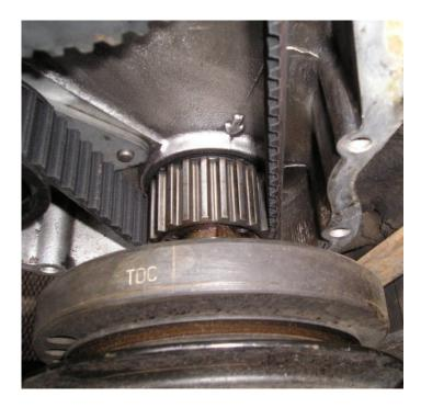
I should have put this in earlier, but I didn't refer to it much in use. This is obviously the crank damper, at TDC you note that the TDC marks are actually at about 11 o'clock. If you look at the 4th picture on this page you see that a raised seam/line on the timing gear cover plate can be seen running from the crank shaft hole to the horizontal line running across the cover plate. That line at 11 o'clock is what this TDC line will line up with....just so you know!
