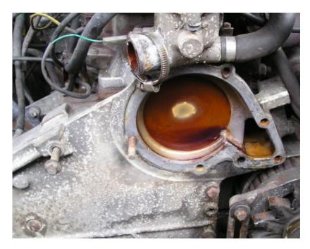
Once that's done, remove the water pump, and move the two hoses too it out of the way.
