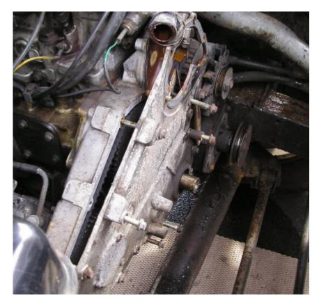
Its got a gasket on it, so it may take some pressing off. Note that my crank damper is removed. You may need to use a puller to remove this, but mine was loose after I undid the bolt. It has a woodruff key that signifies the crank is at TDC.
